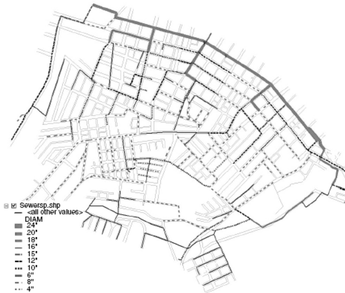
Figure 9.2 A sewer system map. Above: without attribute classification and symbology; below: with attribute classification and symbology for pipe diameter.
